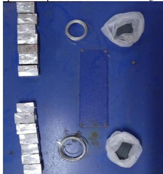
Fig. 2. The ingredients for making the specimens which were used in this study. The aluminium 6061 blocks, the magnesium wire, and the SiC particles have been placed left to right in their respective order.
